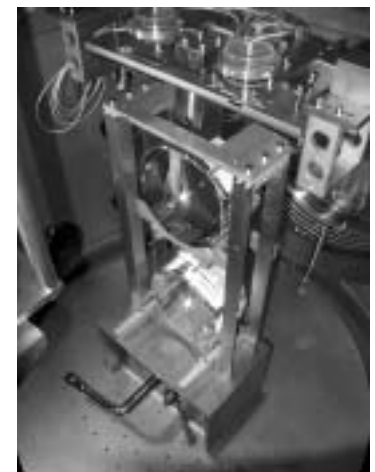
▲ The multiple pendulum suspension system of GEO600. Three two-layer seismic isolation stacks support a structure called rotational stage from which the mirror (test mass) is suspended via two vertical cantilever spring stages and three pendulums for horizontal isolation of the mirror from ground motion. The last pendulum stage is made entirely from fused silica to reduce thermal noise. A reaction pendulum is placed close to the main pendulum to allow length control of the interferometer from a seismically isolated actuator.
