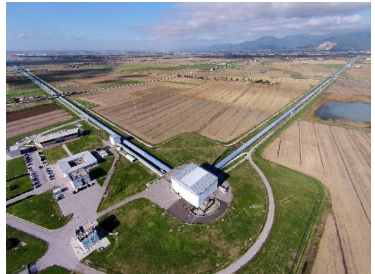
Aerial view of the Virgo gravitational-wave detector, situated at Cascina, near Pisa (Italy). Virgo is a giant Michelson laser interferometer with arms that are 3 km long. (Image credit: Nicola Baldocchi / Virgo Collaboration)
